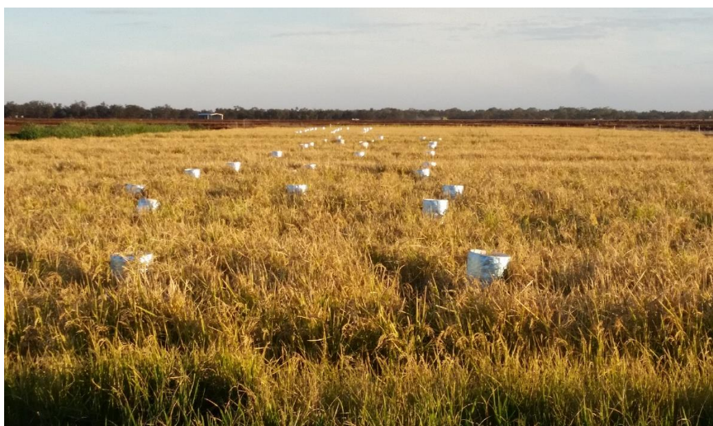
Figure 2. Static chambers positioned in plots with external reflective foil to minimise heat buildup within the chamber during the 1.5 hr incubation period
