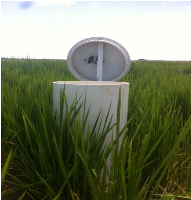
Figure 3. Removable battery-operated fan attached to lids to ensure mixing of the air inside the chamber during the 1.5 hr incubation period
