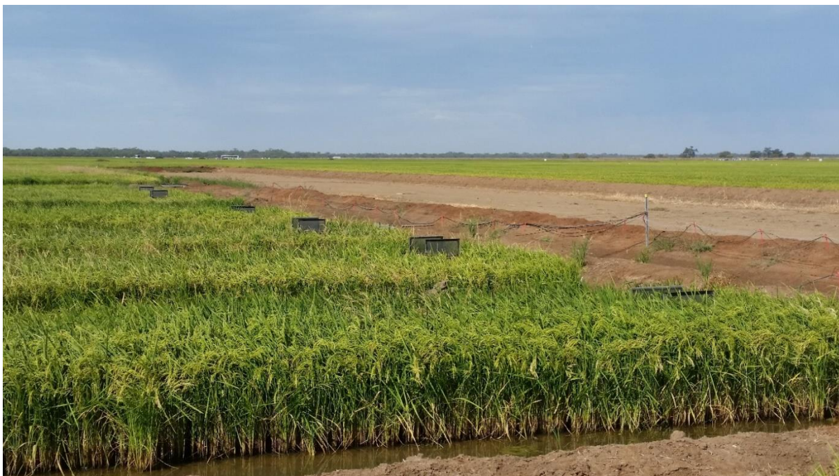
Figure 4. Autochambers used to quantify methane and nitrous oxide emissions in the 2015-16 season
